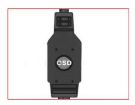
To select the video output mode push and hold the OSD joytick in for 5 seconds, do this several times until desired output is selected. Output mode will diplay on screen when format is changed.
