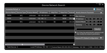
9. Under Modify network parameter, change the first 3 DIGITS (OCTETS) OF THE IP ADDRESS TO MATCH THE NETWORK SCHEME FROM STEP 5 ABOVE. THE LAST OCTET WILL BE A DIFFERENT NUMBER, YOU MUST CHOOSE AN IP ADDRESS THAT IS AVAILABLE ON THE NETWORK TO PREVENT A CONFLICT. Use the PING command in the command prompt to find and available IP address.
