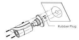
④ Bracket adjustment: Before adjusting the bracket, preview the placement view of the camera on a monitor. If you need to adjust the angel, loosen the fixed ring. Adjust the view angle of the camera until you reach the desired placement view.
