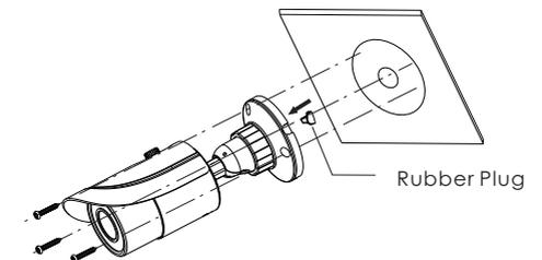
④ Bracket adjustment: Before adjusting the bracket, preview the placement view of the camera on a monitor. If you need to adjust the angel, loosen the fixed ring. Adjust the view angle of the camera until you reach the desired placement view.
