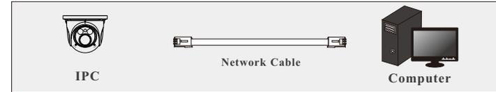
1. connect the IP camera and a Windows computer to a network switch or router
