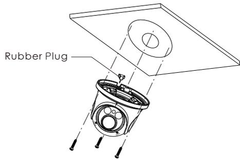
③ Adjust the camera to obtain an optimum angle by loosening the lock screws. Before adjustment, preview the image of the camera on a monitor. Tighten the lock screws after you finish adjusting the view angle of the camera.
