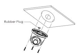
③ Adjust the camera to obtain an optimum angle by loosening the lock screws. Before adjustment, preview the image of the camera on a monitor. Tighten the lock screws after you finish adjusting the view angle of the camera.
