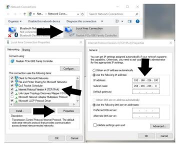
6. After saving your temporary settings on the computer, you can now access the camera using Internet Explorer. In the address bar type: http://192.168.226.201
