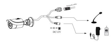
\* 1 It is recommended to install the water-proof cap for network cable connection.
