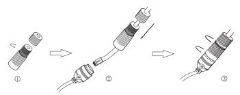
1 Loosen the nut from the main element.
