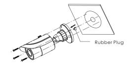
④ Bracket adjustment: Before adjusting the bracket, preview the placement view of the camera on a monitor. If you need to adjust the angel, loosen the fixed ring. Adjust the view angle of the camera until you reach the desired placement view.
