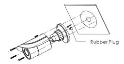
④ Bracket adjustment. Before adjustment, preview the image of the camera on a monitor and then loosen the fixed ring to adjust the view angle of the camera.
