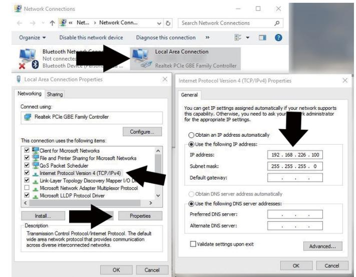
6. After saving your temporary settings on the computer, you can now access the camera using Internet Explorer. In the address bar type:
