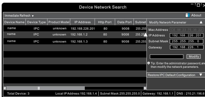
9. Under Modify network parameter, change the first 3 DIGITS (OCTETS) OF THE IP ADDRESS TO MATCH THE NETWORK SCHEME FROM STEP 5 ABOVE. THE LAST OCTET WILL BE A DIFFERENT NUMBER, YOU MUST CHOOSE AN IP ADDRESS THAT IS AVAILABLE ON THE NETWORK TO PREVENT A CONFLICT. Use the PING command in the command prompt to find and available IP address.
