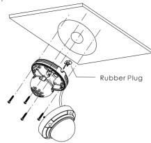
⑤ Three-axis adjustment. Before adjustment, preview the image of the camera on a monitor and then adjust the camera according to the figure below to get an optimum angle.
