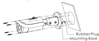
④ Bracket adjustment. Before adjustment, preview the image of the camera on a monitor and then loosen the fixed screws to adjust the view angle of the camera.
