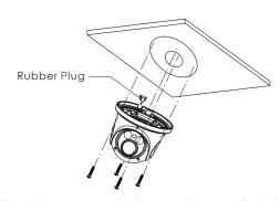
3 Adjust the camera to obtain an optimum angle by loosening the lock screws. Before adjustment, preview the image of the camera on a monitor. Tighten the lock screws after you finish adjusting the view angle of the camera.
