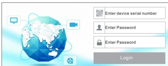
**Device Serial Number:** Click on the menu bar at the bottom of the live interface to check the serial number or go to Start → Settings → Network → Network Status to check the serial number of the NVR).
