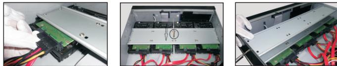
⑦ Install the upper four HDDs and install back the cover.
