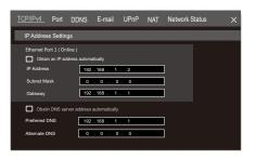
④ Go to Start → Settings → Camera → Add Camera. The NVR will automatically refresh the cameras searched. The IPC which supports the Onvif protocol has be added manually. If the IPC searched is not in the same local network as the NVR, you should select the device and click to modify the IP address.
