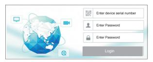
**Device Serial Number**: Click on the menu bar at the bottom of the live interface to check the serial number or go to Start  $\rightarrow$  Settings  $\rightarrow$  Network  $\rightarrow$  Network Status to check the serial number of the NVR).
