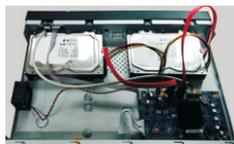
③ Put the HDDs onto the bottom of the device.
