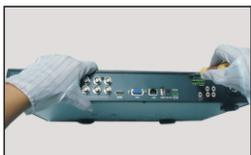
① Loosen the screws on the back.
