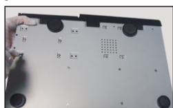
④ Turn over the machine and secure the HDDs with the screws.
