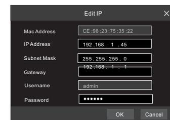
⑤ Checkmark the device you want to add and then click “Add” button. The DVR will automatically refresh the cameras and return to “Edit Camera” interface. “Online” status means the device has been added successfully and you will see the live image. You may select the added device and click button to modify channel, IP address, etc.
