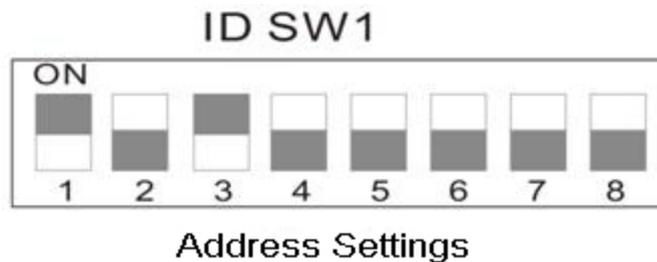
(See illustration above) Turn on the 1st and 3rd (allocated to ON position) and get the binary code 00000101, so the correspondence address is 5.
