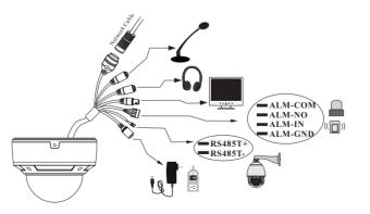
\* 1 It is recommended to install the water-proof cap for network cable connection.
