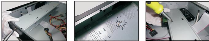
④ Connect the power and data cables and install the other three HDDs according to above-mentioned method.
