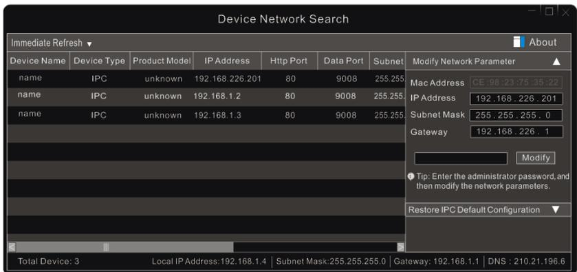
③ Modify the IP address. The **default** IP address of this camera is **192.168.226.201**. Click the information of the camera listed in the above table to show the network information on the right hand. Modify the IP address and gateway of the camera and make sure its network address is in the same local network segment as the computer's. Please modify the IP address of your device according to your local network configuration.
