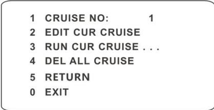
In this interface, by programming presets in cruise list in advance, the system will keep calling those presets at the set time in sequence when executing cruise command so that non-stop monitoring between multiple important positions can be achieved.
