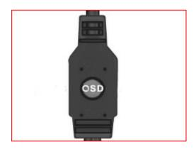
To select the video output mode push and hold the OSD joytick in for 5 seconds, do this several times until desired output is selected. Output mode will diplay on screen when format is changed.
